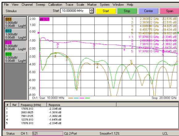
J3 path Insertion Loss vs. Frequency
