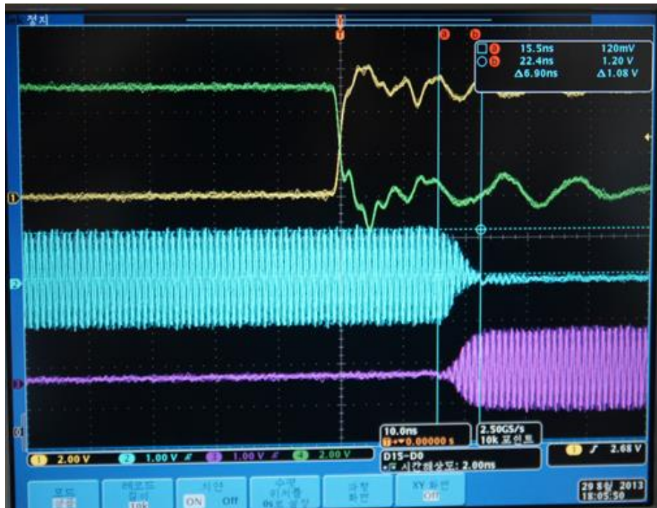
J1-J2 path Falling Time(measured = 6.1 ns)
