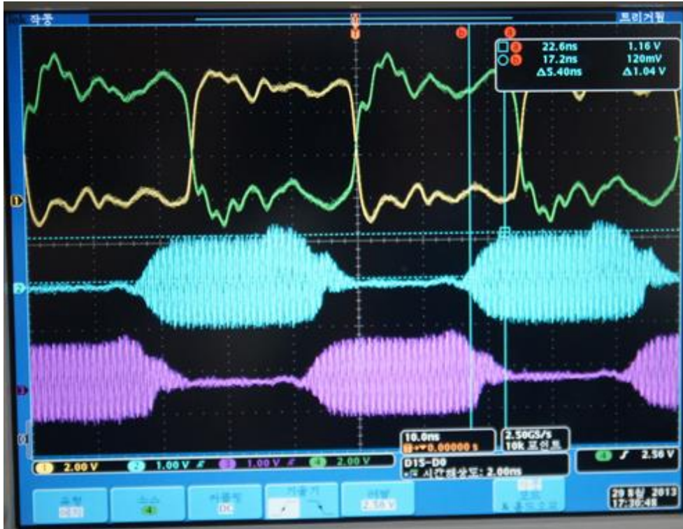
J1-J3 path Repetition Rate(measured @20MHz)
